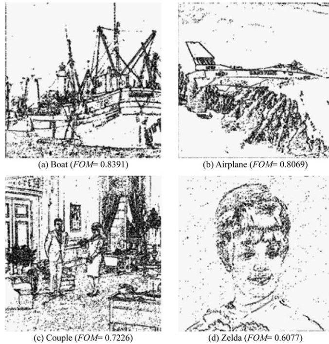
Fig. 14. Four edge maps obtained from the test images by using the proposed approach (a) Boat ( FOM=0.8391 ) (b) Airplane ( FOM=0.8069 ) (c) Couple ( FOM=0.7226 ) (d) Zelda ( FOM=0.6077 ).
