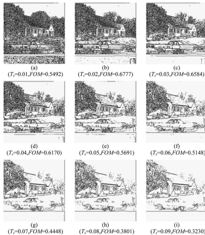
Fig. 15. Edge maps obtained by using the Sobel edge detector with various thresholds (a) ( T_s=0.01, FOM=0.5492 ) (b) ( T_s=0.02, FOM=0.6777 ) (c) ( T_s=0.03, FOM=0.6584 ) (d) ( T_s=0.04, FOM=0.6170 ) (e) ( T_s=0.05, FOM=0.5691 ) (f) ( T_s=0.06, FOM=0.5148 ) (g) ( T_s=0.07, FOM=0.4448 ) (h) ( T_s=0.08, FOM=0.3801 ) (i) ( T_s=0.09, FOM=0.3230 ).
