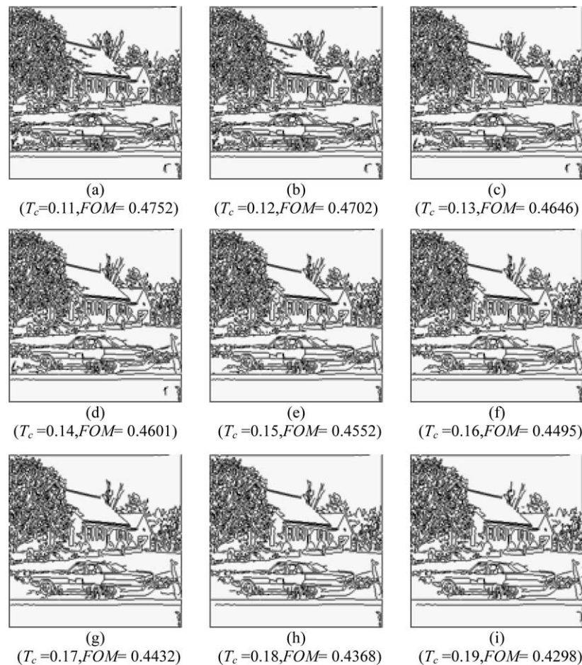
Fig. 16. Edge maps obtained by using the Canny edge detector with various thresholds (a) ( T_c=0.11, FOM=0.4752 ) (b) ( T_c=0.12, FOM=0.4702 ) (c) ( T_c=0.13, FOM=0.4646 ) (d) ( T_c=0.14, FOM=0.4601 ) (e) ( T_c=0.15, FOM=0.4552 ) (f) ( T_c=0.16, FOM=0.4495 ) (g) ( T_c=0.17, FOM=0.4432 ) (h) ( T_c=0.18, FOM=0.4368 ) (i) ( T_c=0.19, FOM=0.4298 ).
