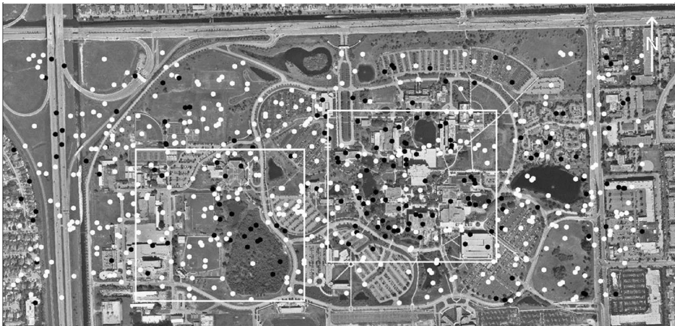
Fig. 4. Aerial photograph for the University Park campus of FIU. Six hundred forty-eight random sample points are also overlain over the photograph. The ground and nonground measurements identified from these samples by the progressive morphological filter are represented by white and black dots, respectively. The white rectangles represent the range of Figs. 5 and 6.
